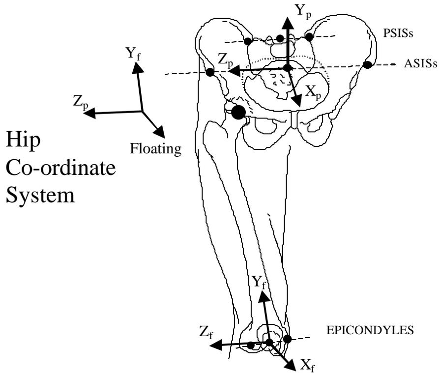
**Figure Legend:** Diagram of pelvis and right femur depicting the coordinate systems.  $X_p$ ,  $Y_p$  and  $Z_p$  are the pelvic orthogonal axes, while  $X_f$ ,  $Y_f$  and  $Z_f$  are the femoral orthogonal axes. The hip coordinate system is derived from the pelvic Z axis ( $Z_p$ ), the femoral Y axis ( $Y_f$ ) and the mutually perpendicular floating axis.
