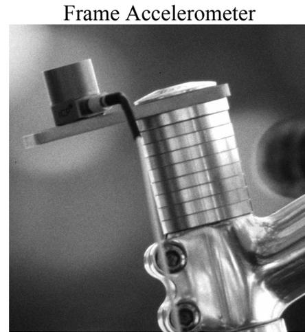
Figure 1: Accelerometer Setup
