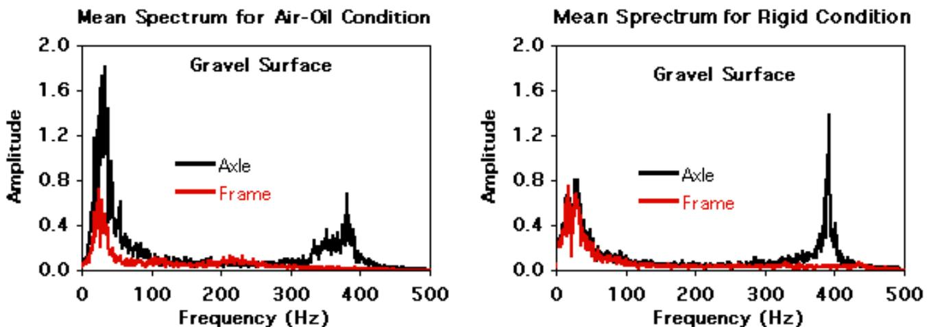
**Figure 2:** Sample Spectral Analysis for Air-Oil and for Rigid Forks
