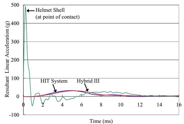
**Figure 2:** For the same impact, the helmet acceleration was approximately 500 g compared to the Hybrid III cg measure of 32 g and the HIT System measure of 33 g.
