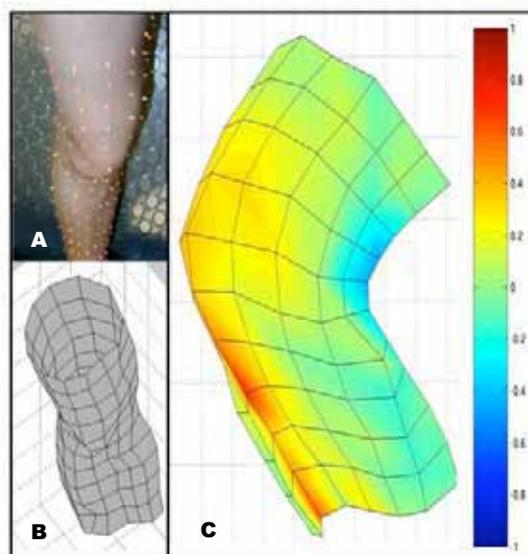
**Figure 1:** A. Raised position trackers covering the leg surface are identified in laser scans and serve as input for a virtual 3D model of the leg. B. Leg reconstruction in initial state, from upper thigh to mid calf, using only the positions of the tracked points. C. Leg reconstruction with 90-degree knee flexion angle, with the magnitude of skin's longitudinal strain overlaid in color.
