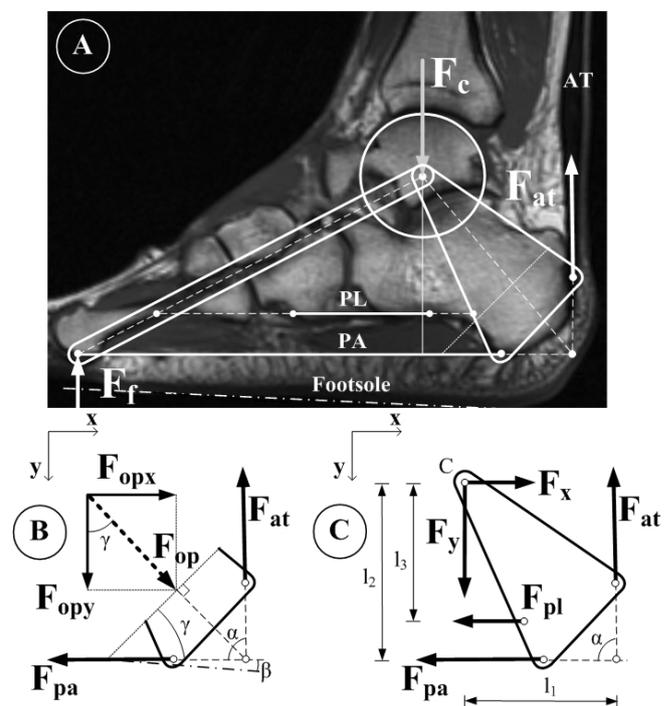
**Figure 2A:** Sagittal T1-weighted MRI study of a foot that is modeled as a system of two trusses, at the apex connected by a hinge and stabilized by two wires representing the plantar aponeurosis (PA) and the long plantar ligament (PL). The ground reaction force at the forefoot ( $F_c$ ) is balanced by the joint contact force ( $F_f$ ) and the Achilles tendon (AT) force ( $F_{at}$ ).
