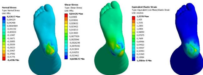
**Figure 2:** Strain, shear stress distribution and plantar pressure during HC.
