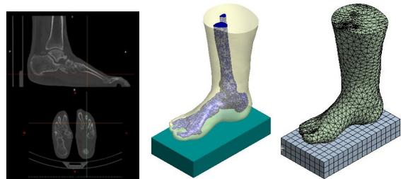
**Figure 1:** CT scan of individual foot (left), 3D foot model after being process in Solidworks® (center) and mesh for Ansys® (right).
