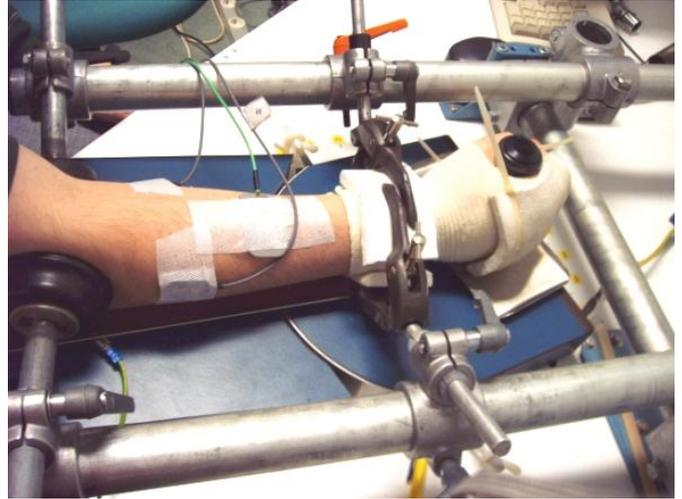
**Figure 1:** Experimental setup showing the elbow and wrist fixation and the wrist perturbator.
