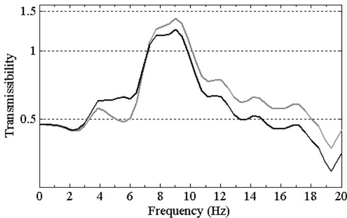
**Figure 1:** Ascending stairs, transmissibility from S1 to T1, before and after correction.
