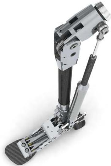
*Figure 3. CAD representation of the prosthetic prototype.*
