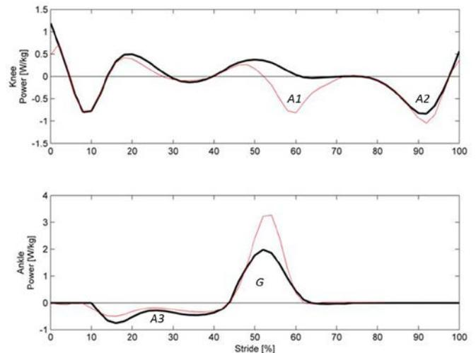
**Figure 1.** The power flow of normal gait for knee (top) and ankle (bottom) joints during one stride (Winter, 1991). The areas  $A1,2,3$  indicate the energy absorption, whereas  $G$  indicates the energy generation. The thick line represents simulation results for an optimized leg prosthesis with required behavior.
