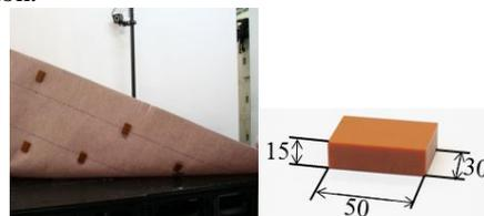
Figure 1: Irregular surface and block. (Back of the carpet.)
