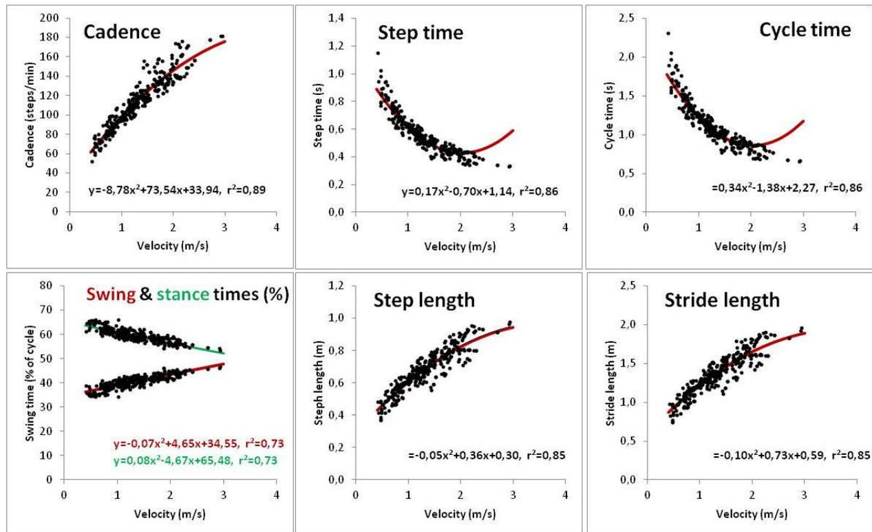
Figure 2: Average second order polynomial regression equations and individual data points for ST parameters.
