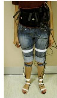
Figure 1. The ambulatory system with a sensor configuration for ankle and foot joints assessment.
