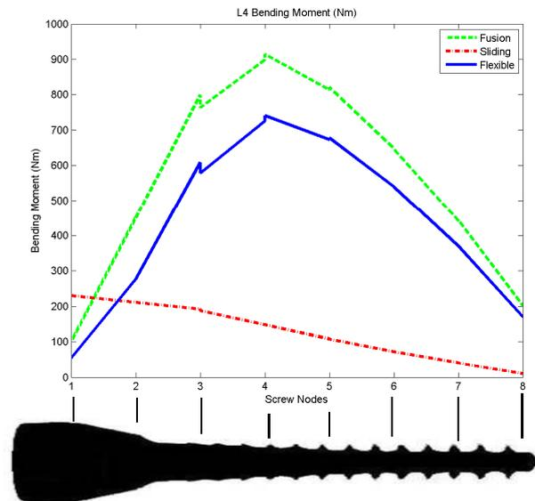
**Figure 1:** Bending moment on a screw for  $17^\circ$  flexion of a L3-S1 spine for different rods designs.
