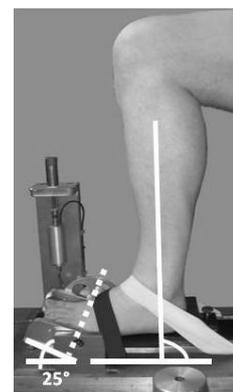
Figure 1: Dynamometer to quantify foot muscle strength.
