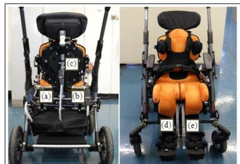
Figure 1: The location of the strain gauge groups
