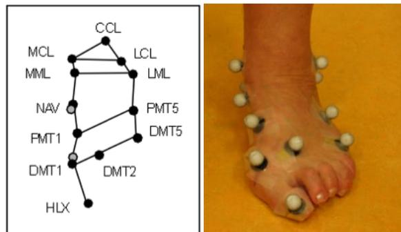
**Figure 1:** Foot and ankle computer model and foot with markers
