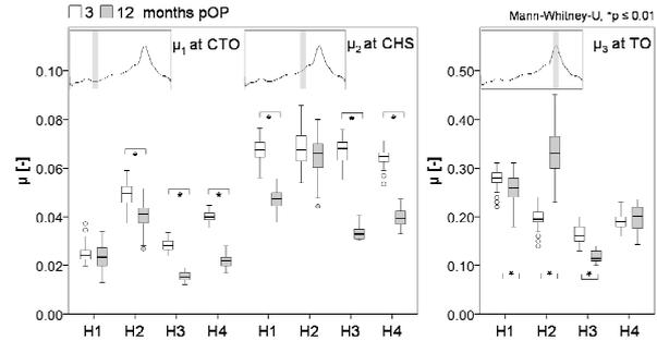
Fig. 2 Coefficient of friction  $\mu$  at 3 instants during the gait cycle. Data from 4 subjects. 3 and 12 months after implantation. CTO = contralateral toe off, CHS = contralateral heel strike, TO = toe off.
