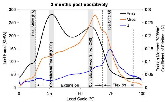
Fig. 1 Patterns of  $F_{res}$  (left scale),  $M_{res}$  and  $\mu$  (right scale) during one cycle of walking. Data from subject H3; 3 months after implantation.
