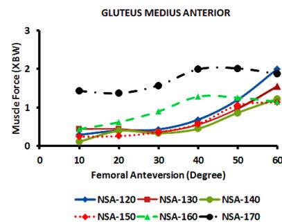
**Figure 2:** Peak gluteus medius (anterior) muscle force as a function of femoral anteversion, at different femoral neck-shaft angles.
