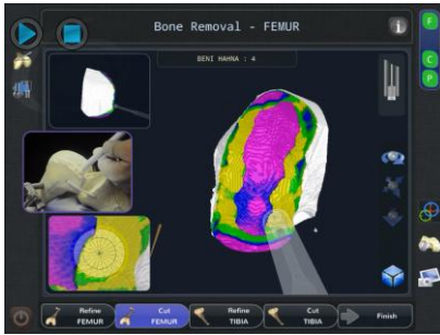
Figure 1: Visual representation of the femur and tibia cutting screen (A) Femur cutting screen prior to cutting (B) Femur cutting screen mid cutting.
