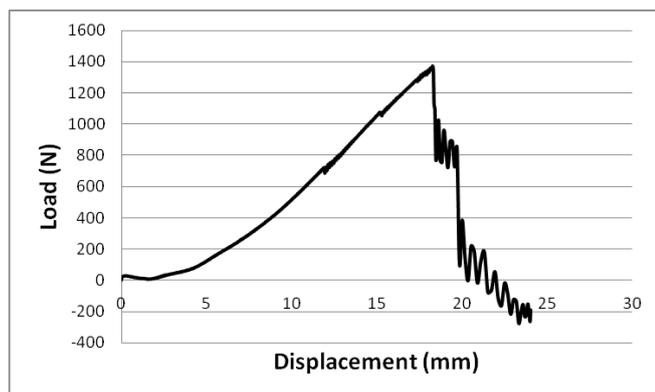
**Figure 2:** Load-displacement curve for TCL tensile test.
