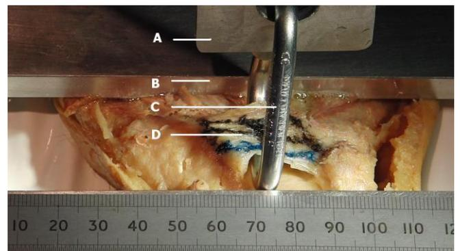
**Figure 1:** Illustration of specimen setup on Instron E10000 (Instron, Bucks, UK) Materials Testing Machine. (A) Steel
