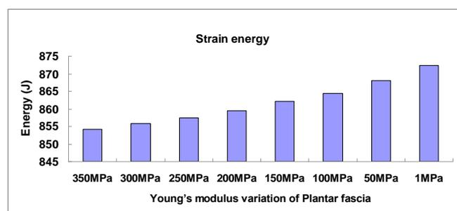
**Figure 4:** The strain energy variation in foot skeletal system
