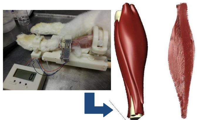
**Figure 1:** (Left) 3D printed MRI rabbit rig with force transducer; (Middle) rabbit finite element model; and (Right) muscle fibers from DTI.
