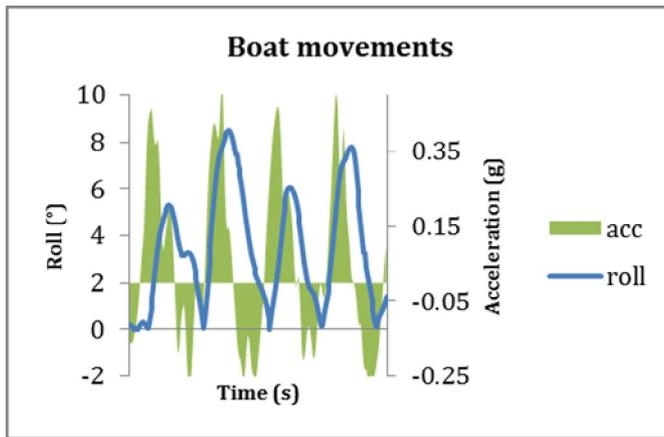
**Figure 2:** Four consecutive strokes showing the boat's forward acceleration and absolute roll.
