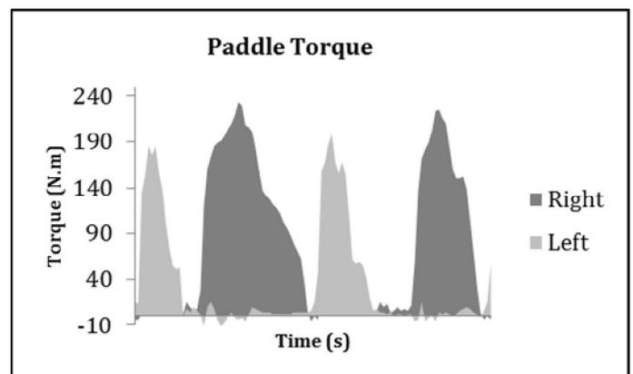
**Figure 1:** Four consecutive strokes showing the magnitude of the torque measured by the strain gauges on the instrumented paddle. The shaded area per stroke represents a summary variable for the amount of force applied by the paddler.
