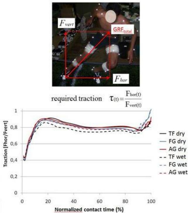
**Figure 1:** Temporal evolution of the required traction, calculated as ratio of the horizontal/vertical component of the ground reaction force [3], executed during the 180° turn by the outward foot; conditions: 3 shoe types (Turf Field, Artificial Grass, Firm Ground) x Wet and Dry AT. Average curves for 11 subjects.
