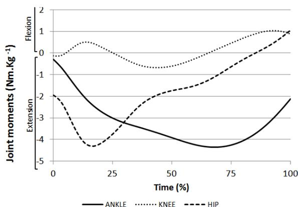
**Figure 2:** Sagittal joint moments of the support leg computed through inverse dynamics.
