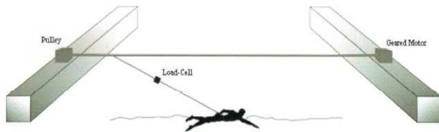
**Figure 1:** Schematic model of the test system.
