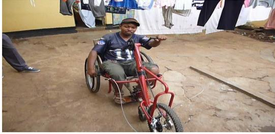
**Figure 2: Final wheelchair tricycle attachment and testing by the user**
