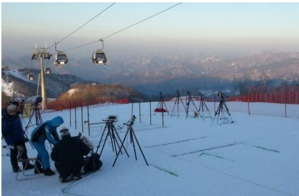
**Figure 1:** Experimental setup on hills using eleven infrared cameras and timing lights.
