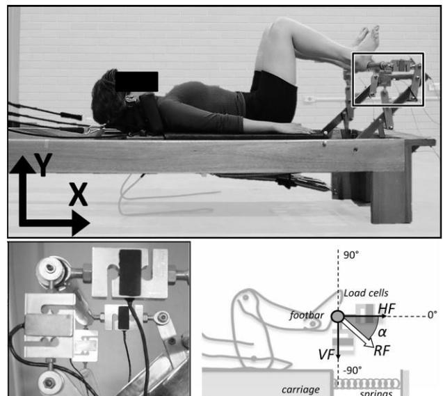
**Figure 1:** Subject performing the Leg Work exercise. The instrumented footbar and schematic figure that represents the main components of the reformer (carriage and springs) and the instrumented footbar.
