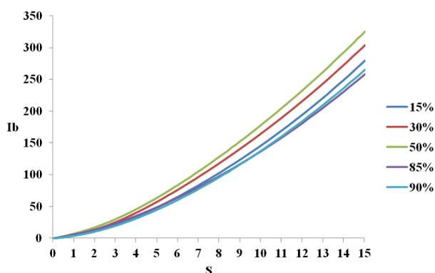
**Figure 2:** Compression force and displacement relationship of a representative baseball sample of each model.
