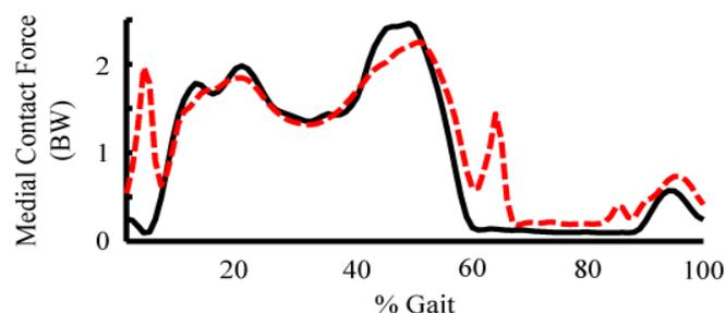
**Figure 2:** Medial contact force for unbraced (black, solid) and braced (red, dashed) gait trials.
