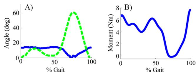
**Figure 1:** A) Brace flexion (dashed, green) and adduction (solid, blue) angles throughout the gait cycle. The brace was deflected roughly 14 degrees in the adduction direction throughout most of stance. B) Abduction moment applied to the knee by the brace throughout gait. The brace applied between 4 and 7Nm of unloader abduction moment to the knee during stance, and was highly sensitive to the brace flexion angle.
