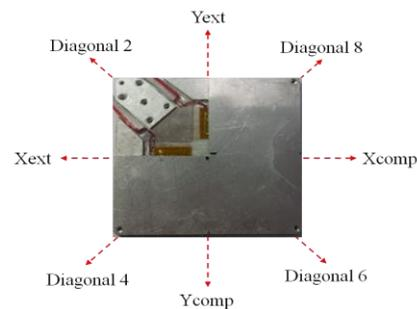
**Figure 1:** Direction of measurement of shear force, Xext: Tensile in the direction of the X axis, Xcomp: Tensile in the direction of the reverse X axis, Yext: Tensile in the direction of the Y axis, Ycomp: Tensile in the direction of the reverse Y axis, Diagonal 2, 4, 6, and 8: Tensile in the direction of the diagonal axis 2, 4, 6, and 8, respectively
