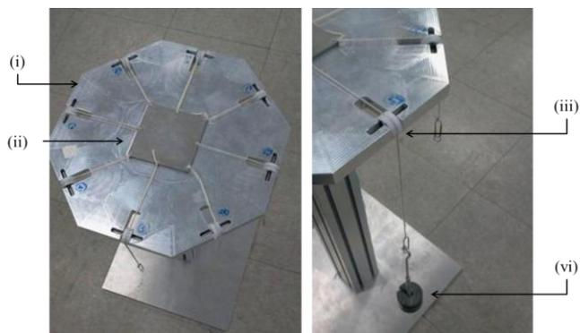
**Figure 2:** The validation and calibration apparatus (i) base plate (ii) sensor fixing unit (cover plate and lower fixing plate) (iii) pulley unit (wire and guide groove) (vi) standard weight
