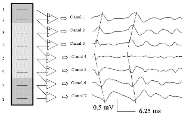
**Figure 1:** Propagating potential in the short head biceps brachialis muscle (elbow flexion to 90°; linear array of eight electrodes of silver of 10 mm length and 1 mm diameter, 10 mm distance between electrodes in bipolar configuration). Dotted lines illustrate the propagation of action potentials of the motor units. The innervation zone is in the region of the
