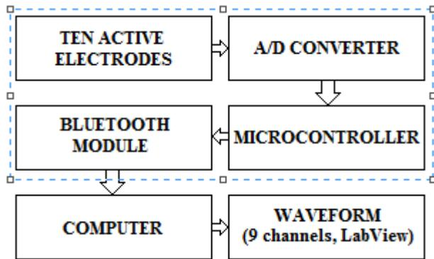
**Figure 2:** Block diagram of the linear electrode array: the developed hardware is in a package containing ten electrodes, analog / digital converter, microcontroller and Bluetooth module.
