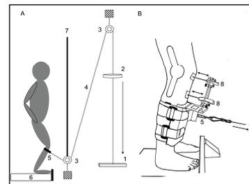
**Figure 1:** Schematic drawing of the experimental setup. A: Experimental setup, B: Measurement system | 1: stopper, 2: falling weight, 3: pulley, 4: steel rope, 5: force transducer, 6: force
