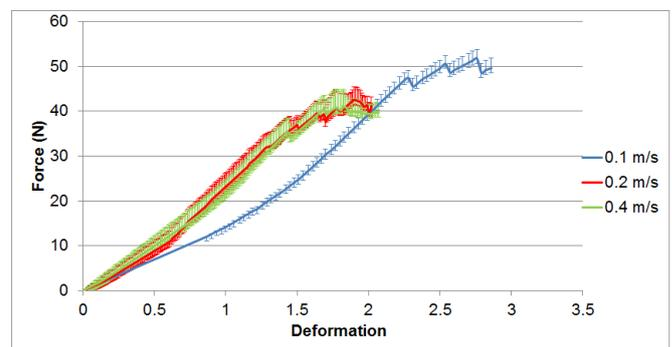
Figure 2: PCL Force/Deformation curves depending on the used crosshead speed.
