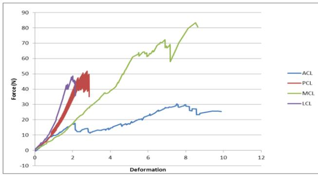
**Figure 3:** Ligaments Force/Deformation curves depending on the same used crosshead speed.
