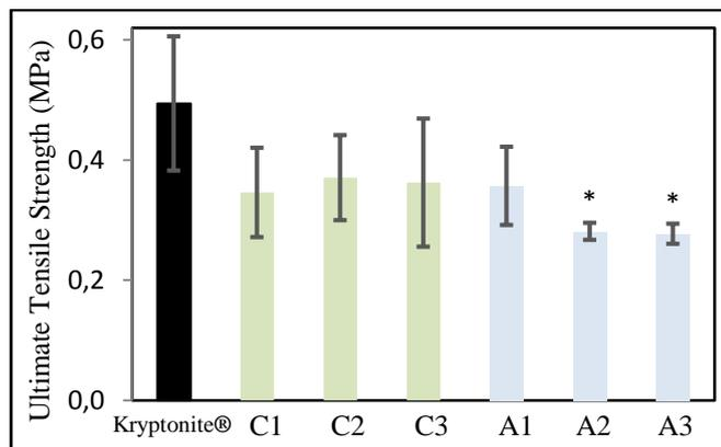
Figure 3. Results for TT90 for adhesive based on chitosan and alginate compared with Kryptonite®, Significance difference (\* $p < 0.05$ ). Error bars of one standard deviation.
