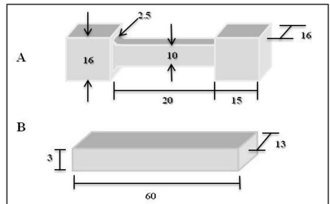
Figure 2. Specimens of A) TT90 and TT45 and, B) 3PFT. All measurements are in mm.
