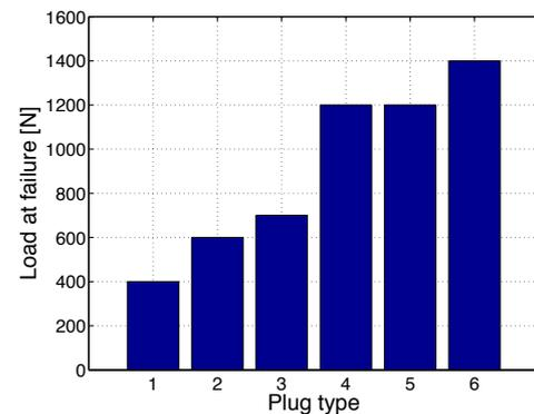
**Figure 1:** Mean failure load of the tested specimen (1-unlocked, 2-Synthes® End Caps, 3-Hofer® Plug 3mm, 4-Hofer® Plug 3.5mm, 5-Hofer® Fix Plug, 6-Hofer® Twin Plug)
