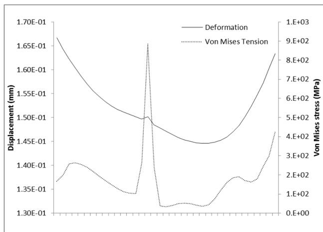
**Figure 2:** Equivalent stress and displacement in fossa component.
