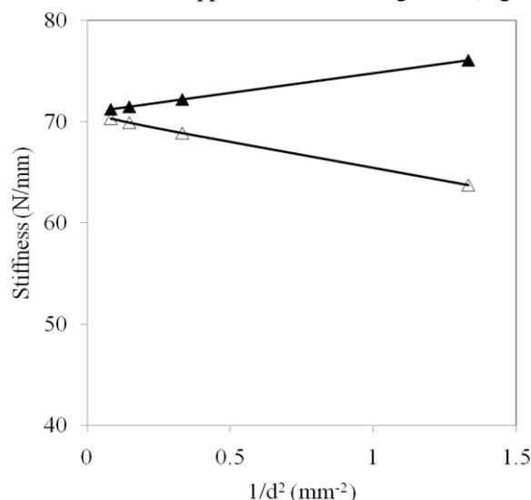
**Figure 3:** Computational results for beams with a void fraction of 8.2% and normalized void radius of 0.12. Continuous beams with a micropolar size effect are shown with solid triangles. Corrugated beams with surface voids are shown with hollow triangles.
