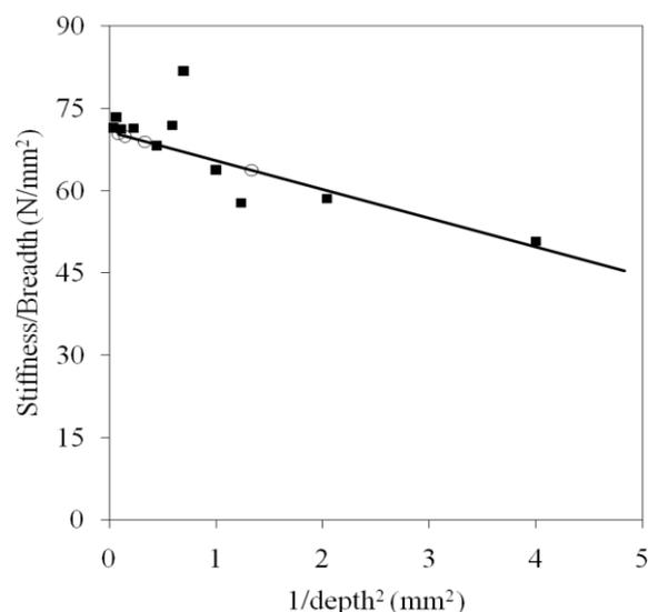
**Figure 4:** The experimental size effect (solid squares) plotted with the numerical size effect trendline produced with a void fraction of 8.2% and normalized void radius of 0.12 (hollow circles).
