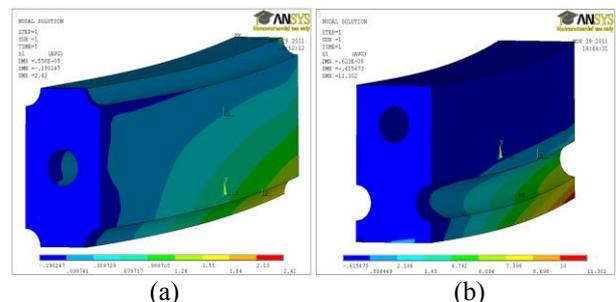
**Figure 2:** The stress distribution for structural units with (a) and without (b) surface voids in three point bending.
