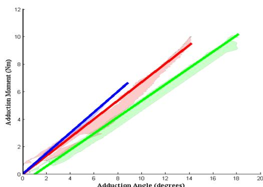
**Figure 2:** Brace abduction moment as a function of brace adduction angle, averaged for each brace for 0-20 degrees of brace flexion to represent the stance phase of gait. Red: “OAActive” (VQ Orthocare), Green: “Unloader Lite” (Ossur), Blue: “Unloader XT” (Ossur).
