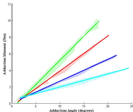
**Figure 3:** Brace abduction moment as a function of both adduction and flexion angles for the “Unloader Lite” (Ossur) knee brace. Decreased stiffness (slope) with increased flexion angle was observed for all three braces. Green: 0-20 degrees flexion angle, Red: 20-40 degrees flexion angle, Blue: 40-60 degrees flexion angle, Cyan: 60-80 degrees degrees flexion angle.
