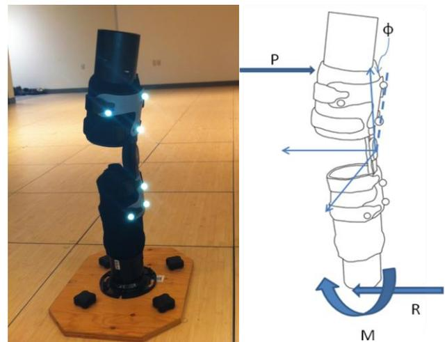
**Figure 1:** Left: VQ Orthocare "OAactive" knee brace rigidly fixed to a six degree-of-freedom force platform with retro-reflective motion tracking markers applied to thigh (top) and shank (bottom) segments. Right: Illustration of measured reaction force,  $R$ , and reaction moment,  $M$ , brace adduction angle,  $\phi$ , and applied load,  $P$ . Flexion and internal rotation deflection angles are not shown.
