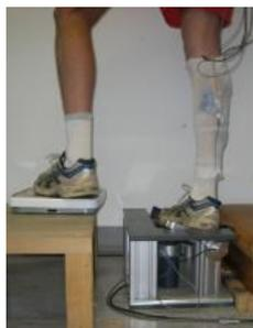
Figure 1: Ankle injury simulation during single leg stance by a custom made tilt platform (University of Freiburg, Germany) to induce 25° of Inversion and 15° of Plantarflexion.
