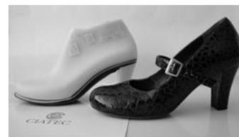
**Figure 1.** Shoe last and prototype footwear
