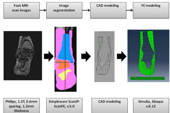
**Figure 1:** The figure shows the workflows of the development of a FE model of the hindfoot.
