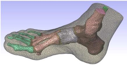
**Figure 3:** 3D mesh of the whole foot and ankle with bones grouped into segments.
