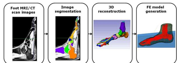
Figure 2: Workflow to obtain the 3D FE foot and ankle models.
