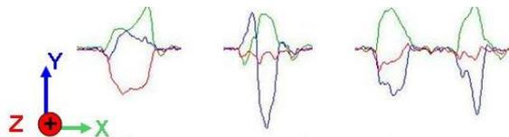
Figure 4. Variation in reaction force-time curves during different WC propulsion cycles also serve to characterize aspects hand/rim interaction including pull up on the rim (+blue), inward push on hand rim (-red), push (+green).
