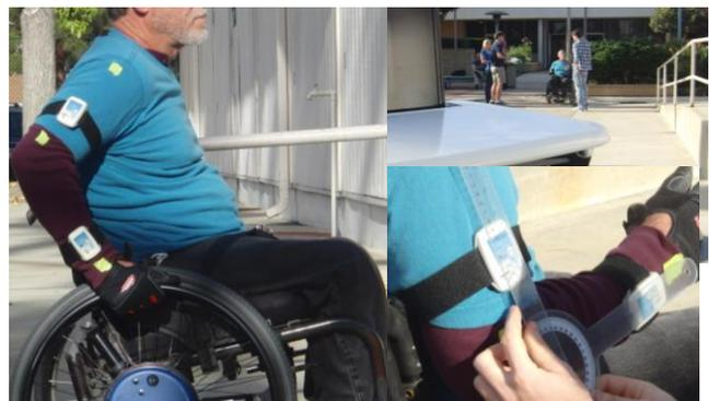
Figure 1. Wearable sensors secured to the upper arm, forearm, and WC were used to monitor segment and WC kinematics. Sensor signals were transmitted via Bluetooth to portable laptop computers.
