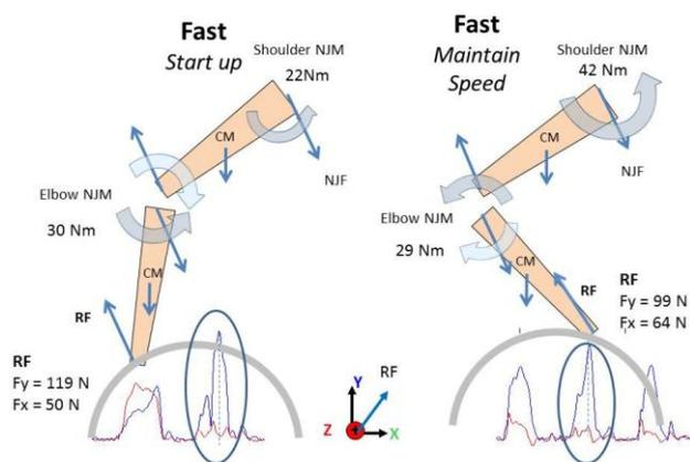
Figure 3. Free body diagrams reflecting the orientation of the reaction force relative to the upper extremity segments at the time of peak push (vertical line) during the fast condition during start up and maintaining speed. Exemplar reaction forces resultant  $RF_{xy}$  (blue),  $RF_z$  (red) time curves during different cycles are also provided to illustrate the variability between cycles and phases.
