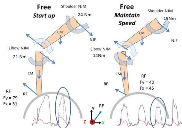
Figure 2 Free body diagrams reflecting the orientation of the reaction force relative to the upper extremity segments at the time of peak push (vertical line) during the free condition during start up and when maintaining speed. Exemplar reaction forces resultant  $RF_{xy}$  (blue),  $RF_z$  (red) time curves during different cycles are also provided to illustrate the variability between cycles and phases.
