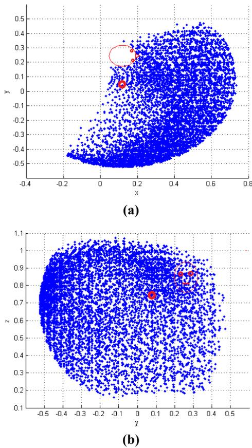
**Figure 2:** working space of human arm in presence of the assistive device: (a) top view, (b) front view where red circles show the position of head and shoulder joint.
