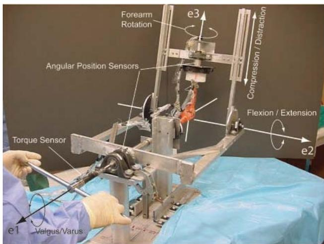
**Figure 1:** Four-degrees-of-freedom (flexion/extension, varus/valgus, forearm rotation, and compression/distraction) loading system. The device allows positioning of the elbow at various degrees of flexion while loading the elbow in valgus and measuring the applied torque, valgus angulation, and forearm rotations.
