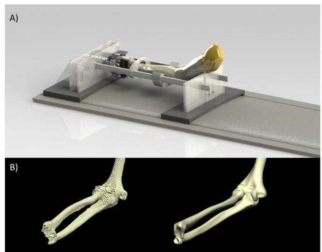
**Figure 1:** The MRI compatible jig used to position and constrain the forearm during scanning (A). Segmented data clouds representing the humerus, ulna and radius, and the finite element model of these bones (B).
