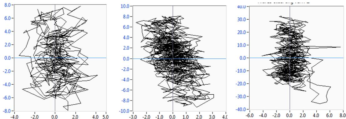
**Figure 2:** Steering angular velocity with respect to bicycle frame in x- (heading) and z-(vertical) direction at a. normal cycling, b. slow cycling, c. cycling while turning head 3 times.
