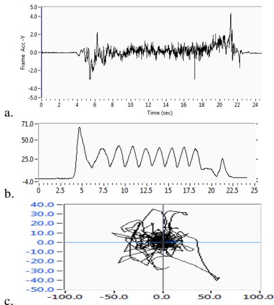
**Figure 1:** a. Lateral acceleration of the frame and b. Upper leg orientation as function of time; c. Upper body angular velocity in x- and z- direction. During: getting on, normal straight cycling, and getting off.
