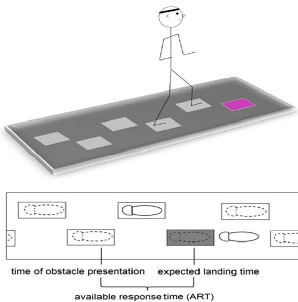
**Figure 1:** Illustration of the experimental setup and ART. Subjects should step onto projected patches of light unless a patch changes color to purple, in which case they should avoid it.
